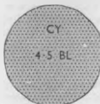
End view showing markings on closing disc
